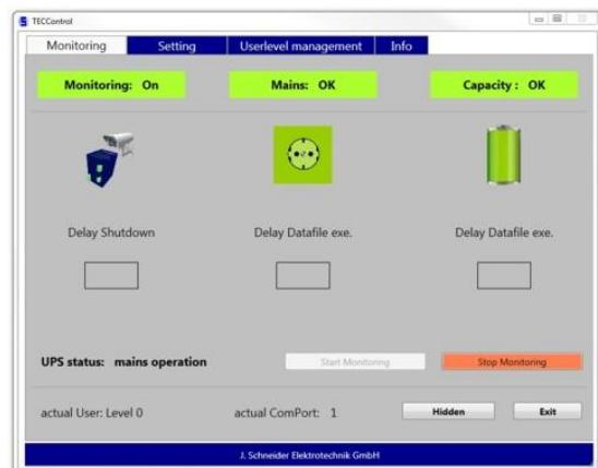
The **TECCcontrol**-Software automates the system-shutdown at power failure and the controlled system-restart after power recovery.
