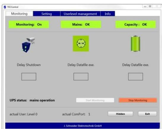
The **TECControl**-Software automates the system-shutdown at power failure and the controlled system-restart after power recovery.
