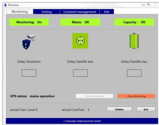
The TECControl -Software automates the system-shutdown at power failure and the controlled system-restart after power recovery. Please ask for further information!
