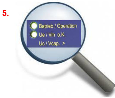
5. Switch on the power supply. The C-TEC is charging. The LEDs „Betrieb/Operation“ and „Ue/Vin o.k.“ illuminate
