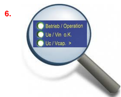
6. C-TEC is completely charged. The LEDs „Betrieb/Operation“, „Ue/Vin o.k.“ and „UC/Vcap. >“ illuminate
