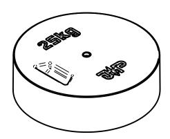
On synthetic roofing membranes a support plate for concrete bases is necessary.
