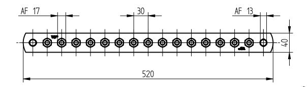
Suitable for the connection in explosive atmospheres in zones 2/22. The terminals of the equipotential bonding bar are secured against self-loosening by a spring washer according to DIN EN 62305-3 Supplement 2.
