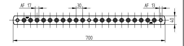
Suitable for the connection in explosive atmospheres in zones 2/22. The terminals of the equipotential bonding bar are secured against self-loosening by a spring washer according to DIN EN 62305-3 Supplement 2.
