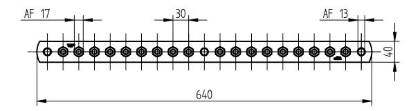
Suitable for the connection in explosive atmospheres in zones 2/22. The terminals of the equipotential bonding bar are secured against self-loosening by a spring washer according to DIN EN 62305-3 Supplement 2.
